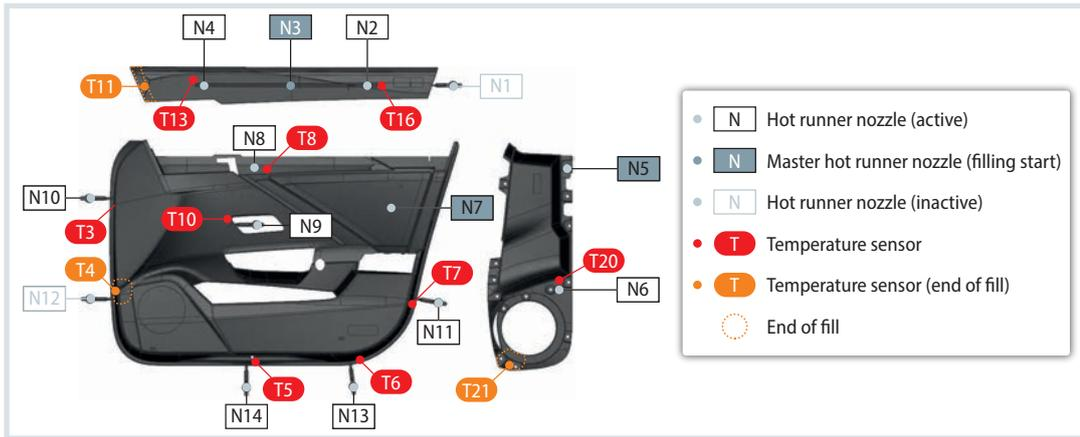
**Fig. 2.** Nozzle and sensor positions in the test mold. The nine red temperature sensors are used for automatic cascading with Priamus Fillcontrol Switch. The three orange sensors monitor the respective flow path ends. © Barnes Molding Solutions
