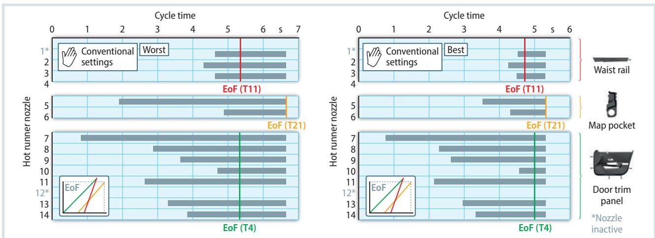
**Fig. 3.** Diagram of the flow path end for the manual set-up of a cascade in a family mold. Even after manual optimization by the setter (right), a filling time difference and thus the risk of overfilling two cavities remains.
