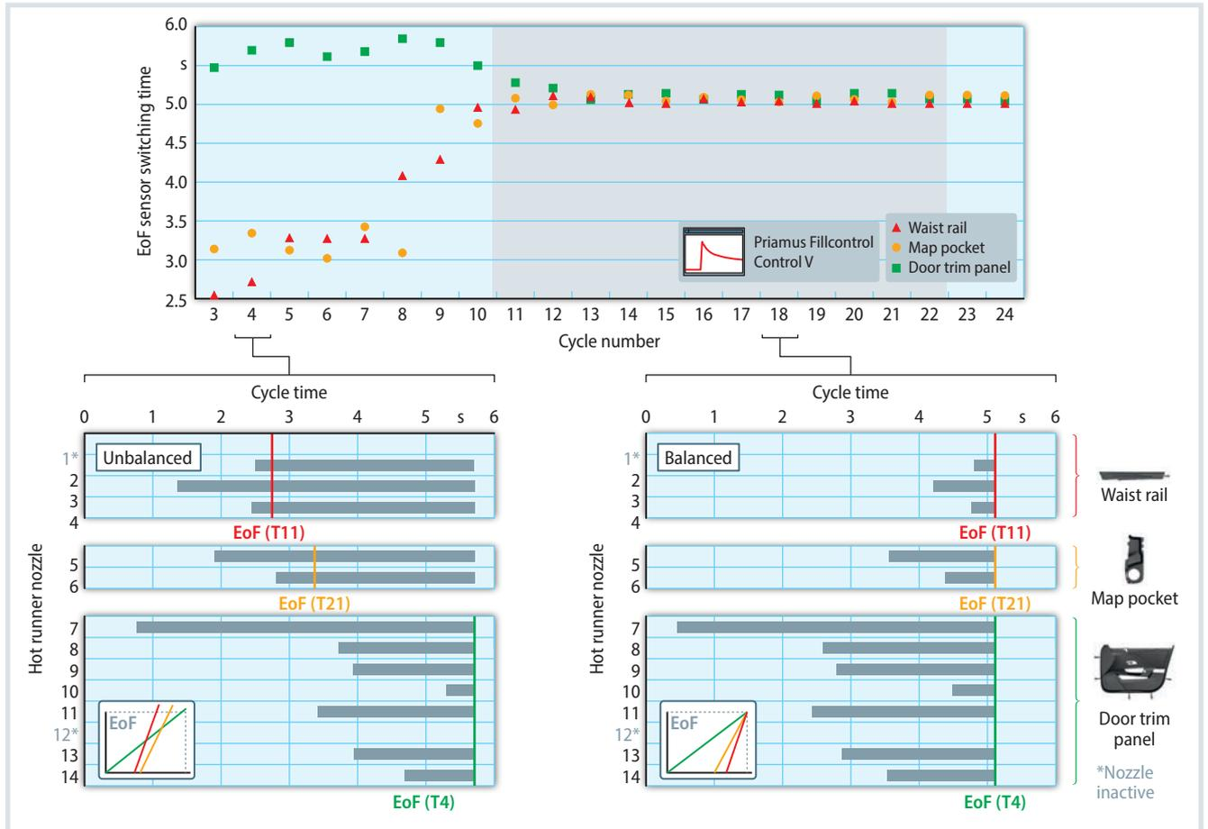
**Fig. 4.** With Priamus Fillcontrol Control V, the filling time differences of the individual cavities are synchronized further with each cycle. The figure shows the switching times of the temperature sensors at the respective flow path ends of the individual cavities. Source: Barnes Molding Solutions, Simon
