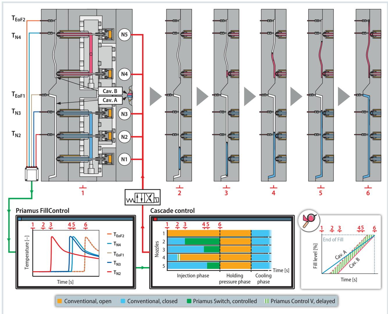
**Fig. 1.** Automatic cascade control using temperature sensors and Priamus Fillcontrol Switch. The family mold shown here has two different cavities and a total of five valve gate nozzles (N1-N5). The different colors of the compound (blue and red) identify the different molded parts.
