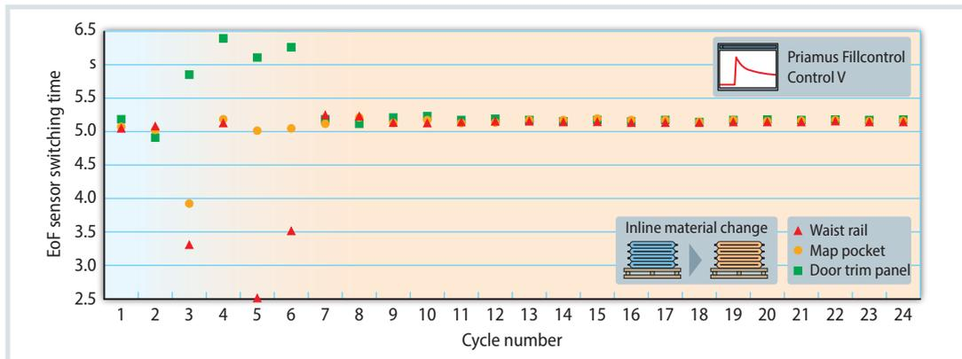
**Fig. 5.** Automatic compensation of fluctuations in the material properties on the example of the inline change to recompound.
